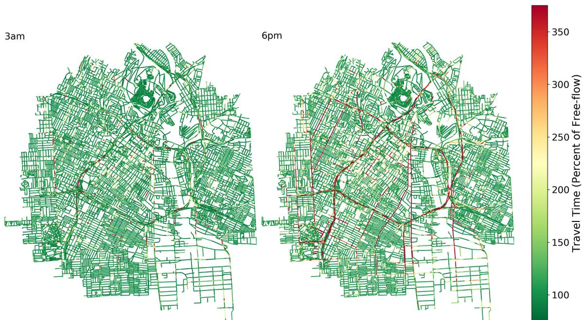
Figure 3: Estimated travel time  $t$  as a percent of free-flow travel time  $f$  in downtown LA for off-peak traffic (3am, left) and peak traffic (6pm, right).
