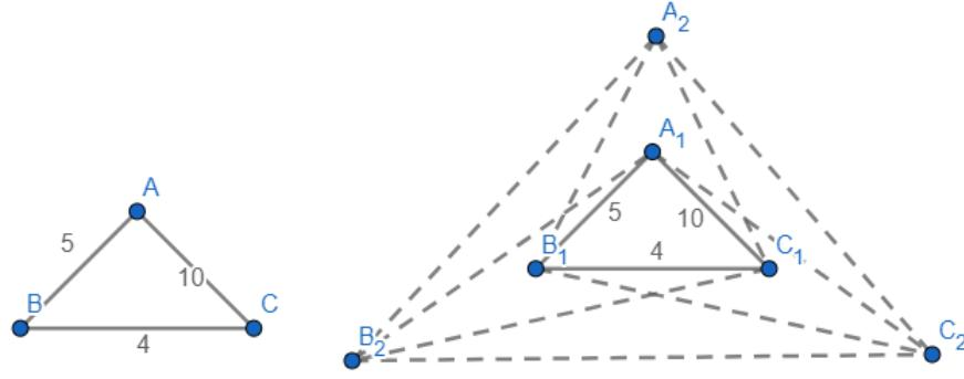
Figure 2. Reduction from a  $b$ -MATCHING to a MATCHING. (Left) Original graph, (Right) Reduced graph for  $b = 2$ .
